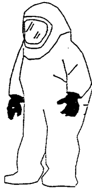
LEVEL A Protection Totally encapsulating vapor-tight suit with full-facepiece SCBA or supplied-air respirator.
